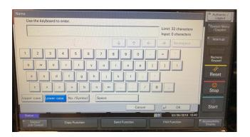
The electronic QWERTY keypad appears when a search key is selected, or when entering an email destination from the scan screen. The keypad is large, and the keys are comfortably spaced. Dedicated "@" and "." Keys are provided on the main screen, but the ability to store extensions (.com, .net) is not supported, nor are typical domains (@gmail.com, @yahoo. com). A subject and three body templates can be stored. A hard keyboard is available as an option.
