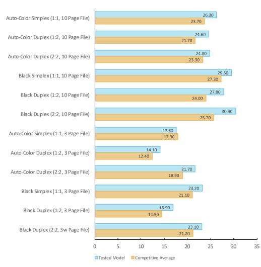
Copy speed is tested using 3-page and 10-page mixed-color and black documents. Buyers Lab obtains the overall speed by averaging the tested speed for each run length (1, 5 and 10 sets).
