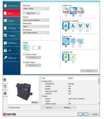
Most typical print job settings are selectable from the Basic tab, including paper type and source, duplex, EcoPrint On/ Off, quantity, and collate sets, although finishing selections such as stapling are programmable from the Finishing tab.
