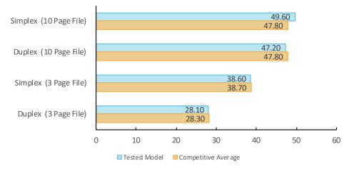
Speed is tested using Buyers Lab's proprietary 3-page and 10-page testing documents. Buyers Lab obtains the overall speed by averaging the tested speed for each run length (1, 5, 10, and 20 sets). The unit was tested using the PCL driver.
