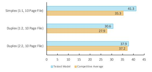
Single-set copy speed is tested using 3-page and 10-page mixed-color and black documents. Timing begins as the start button is pressed, pages are scanned through the document feeder and timing ends when the last page of a single-set of the document exits the device.
