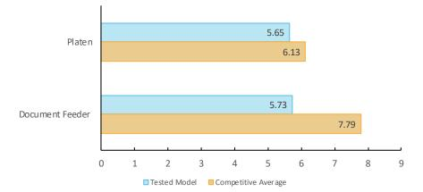
First-copy time is measured as the time it takes for a single copy to completely exit the device when a copy is made from an original placed in the document feeder and on the platen.
