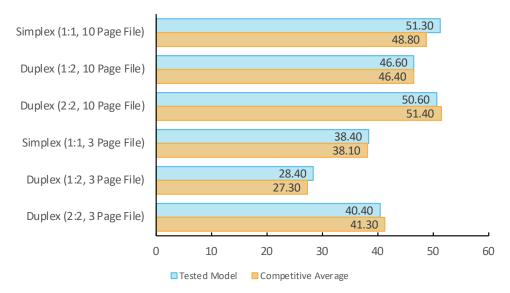
Copy speed is tested using 3-page and 10-page mixed-color and black documents. Buyers Lab obtains the overall speed by averaging the tested speed for each run length (1, 5, 10, and 20 sets).
