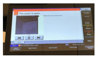
Users are also presented with an animated video to help clear misfeeds; users can let the video play or scroll through step by step using the arrows at the control panel.
