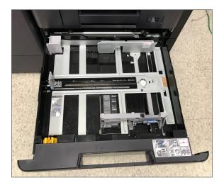
Both length and width guides slide in sync when adjusting paper size in the drawers and have blue locking tabs for easy view. The drawers also feature easy-to-see limit indicators for standard paper, envelopes, and small sizes. The soft close drawers make for no slamming of cassettes, and also pull out far enough for easy access in case of a misfeed.
